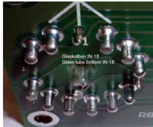
Figure 23 - After soldering the pins
