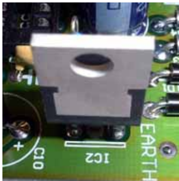
Figure 15 - Proper mounting of IC2
