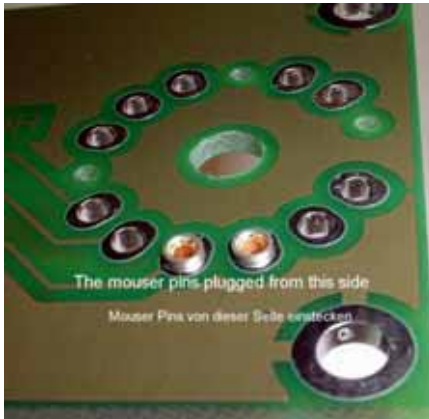
Figure 21 - Top of the PCB with 2 pins in place
