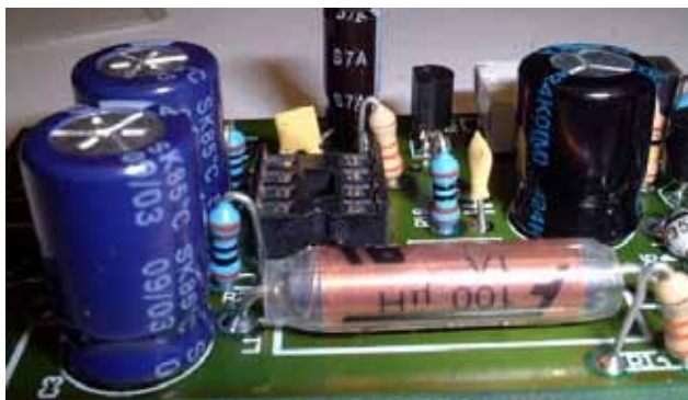
Figure 11 - Proper mounting of the large capacitors
