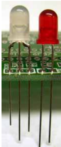
Figure 14 - Dual Color LED D30 DCF77 signal quality or blinking colons and status LED
