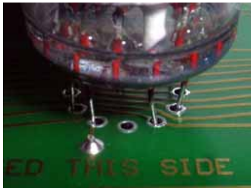
Figure 27 - Make sure the tube is straight.
