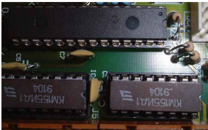
Figure 18 - Proper mounting and orientation of the ICs – see the notch or the dot on the IC
