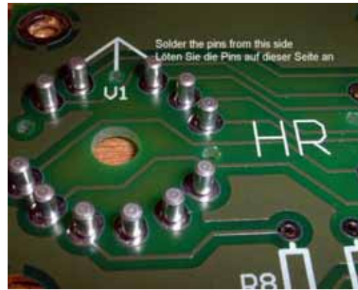
Figure 22 - Bottom of the PCB, before soldering
